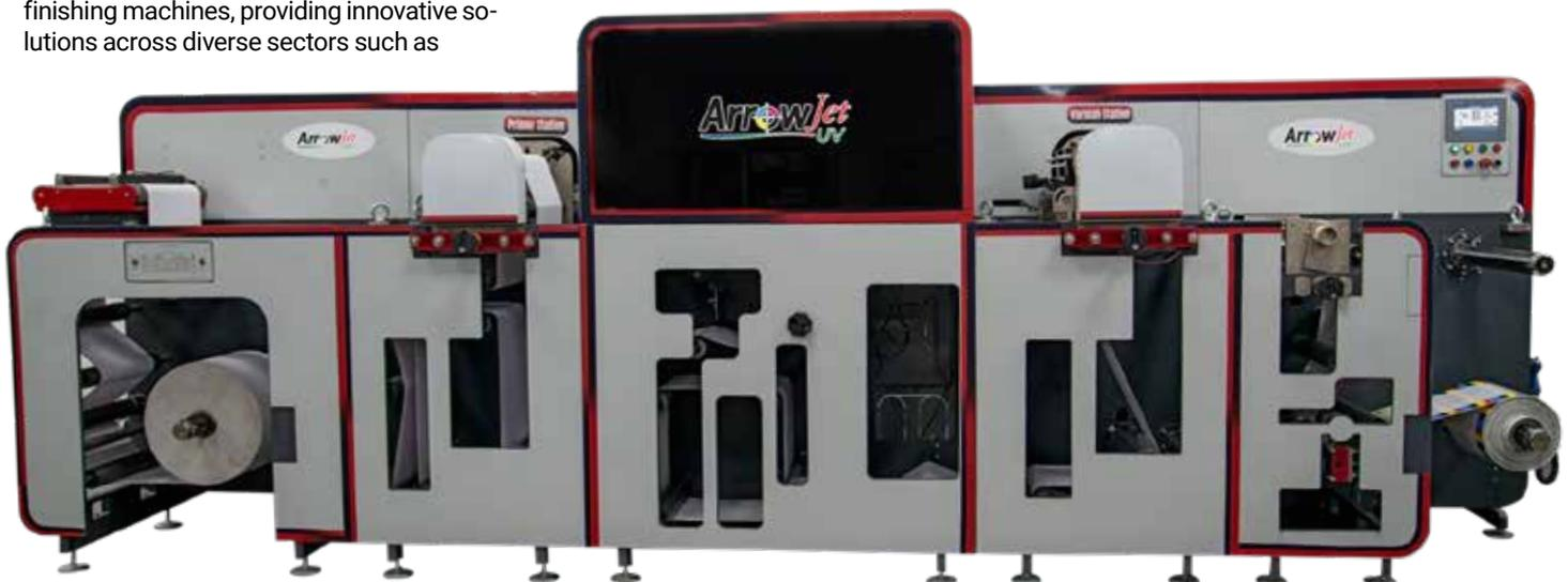
*The ArrowJet UV Machine, powered by Megnajet's HiValve system, delivers high-performance digital printing for labels and packaging.*
